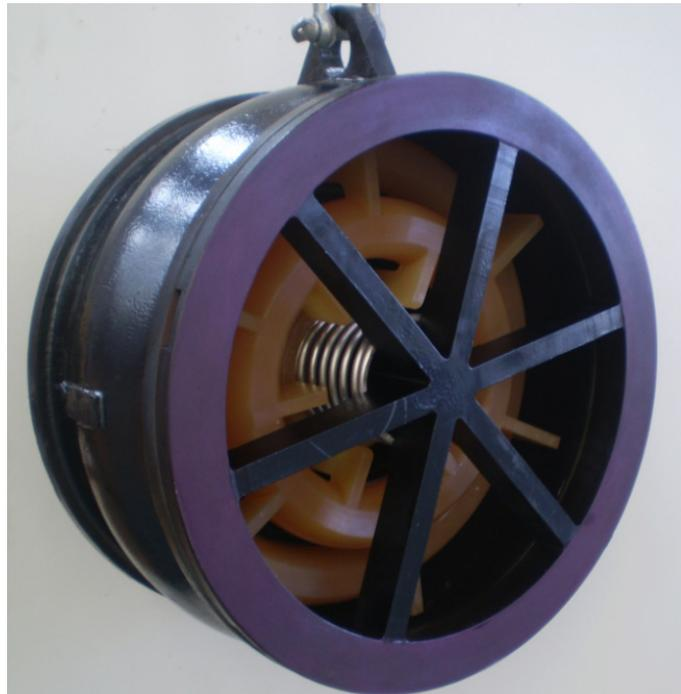
equipment is the material used in the moving part of the valve. This material has specific weight near the fluid, thus balancing the Archimedes thrust effect on the shutter, minimizing the effects of its own weight on the opening / closing of the valve.
